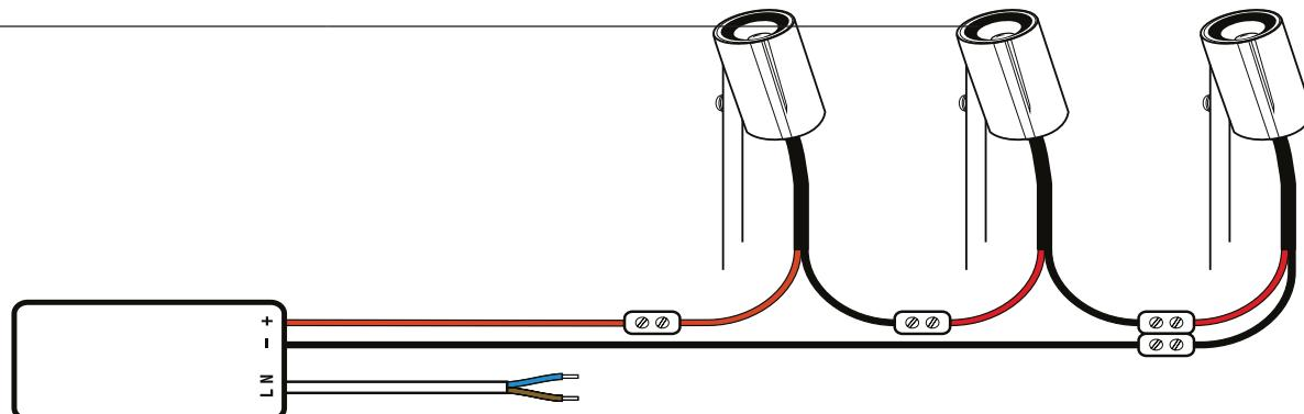
TYPICAL WIRING. NOTE SERIES CONNECTION - INTO POSITIVE, OUT OF NEGATIVE INTO POSITIVE ETC. Easy connection boards are available as an alternative.
